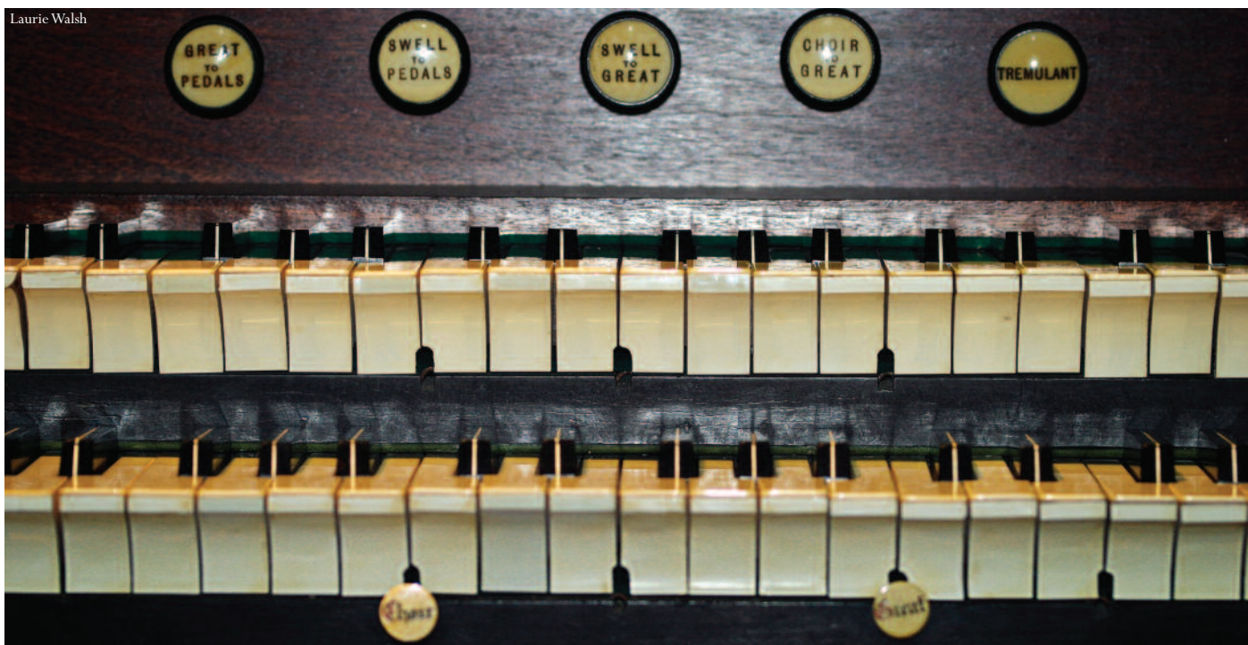
Keyboards, showing missing pistons
