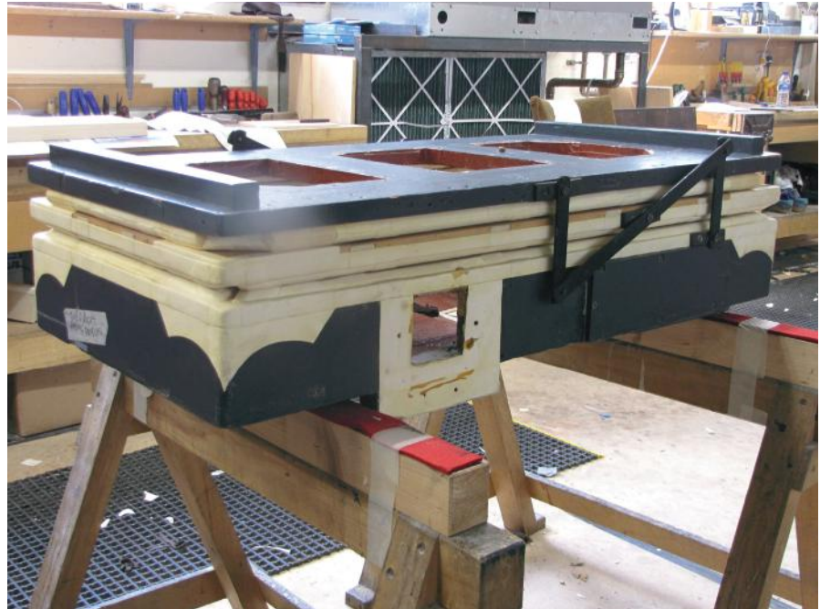
▲ Work included (l) restoring ebony caps to the pedal sharps, to the Willis pattern; a central task (r) was releathering many of the reservoirs
