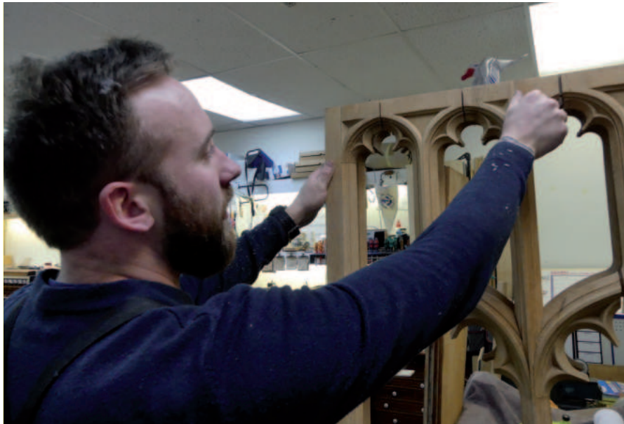
▼ Work on the York instrument continues: (clockwise, from top right) Darren Bingham repairs splits in casework panelling; Csaba Farkas fits counterbalances to a restored reservoir; David Roskelly works on mechanical stop action; the empty case, with front pipes in the background; assistant foreman Tim Bennett assesses an Open Wood ventill
