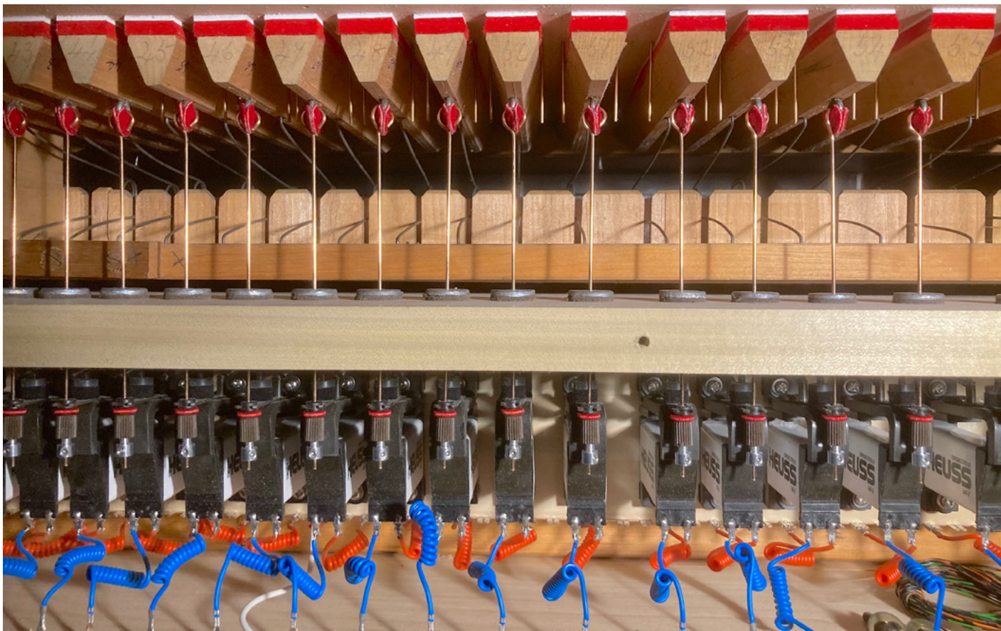
Image 4 | Restored Great soundboard fitted with pull-down magnets
