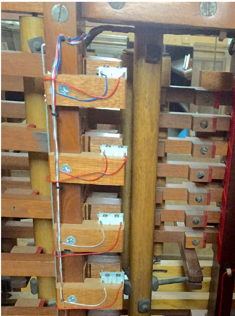
Image 3 | Electrification of the stop action, leaving all mechanical parts in place for composition pedals
