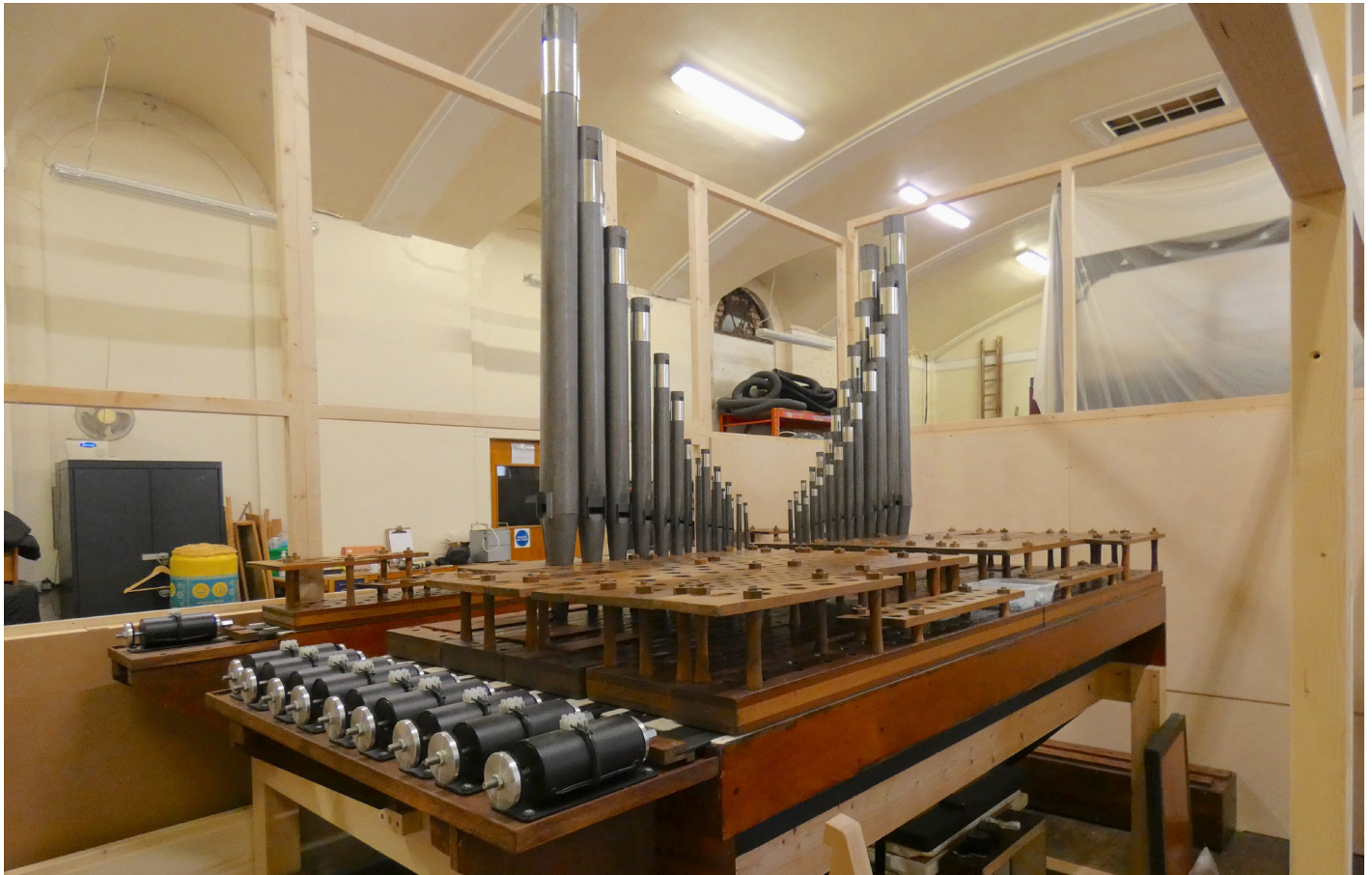
Image 3 | Echo soundboard within swell box under construction at David Wells Ltd
